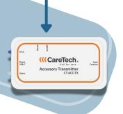
Power on the transmitter with the switch on the top of the device. Check the colour that flashes when powering on. If the LED flashes **red**, proceed to step 3.
