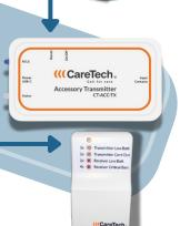
Hold the pair button on the receiver for 4 seconds or until the LED on the front **flashes green**. The LED will blink for 3 seconds. While the LED is still blinking, press the reset button on the transmitter.
