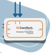
If the LED flashes **green**, turn the transmitter off, then while holding the reset button, turn the transmitter back on. The LED will change to **red** once you let go of the reset button.
