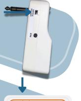
Power on the receiver with the switch on the side, indicated by the on/off sticker.
